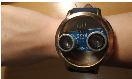
Figure 3: Ultrasonic sensors were integrated into a traditional wristwatch to implement UltraSonic Watch .
